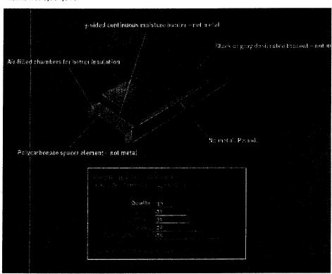
Duralite offers a new level of thermal performance to windows reducing conductivity by up to 45° radical improvement in thermal properties is achieved by eliminating metal and replacing over 60 spacer profile with air. The patented design featuring a unique composite laminating technology the use of metal results in superior thermal and durability performance.
