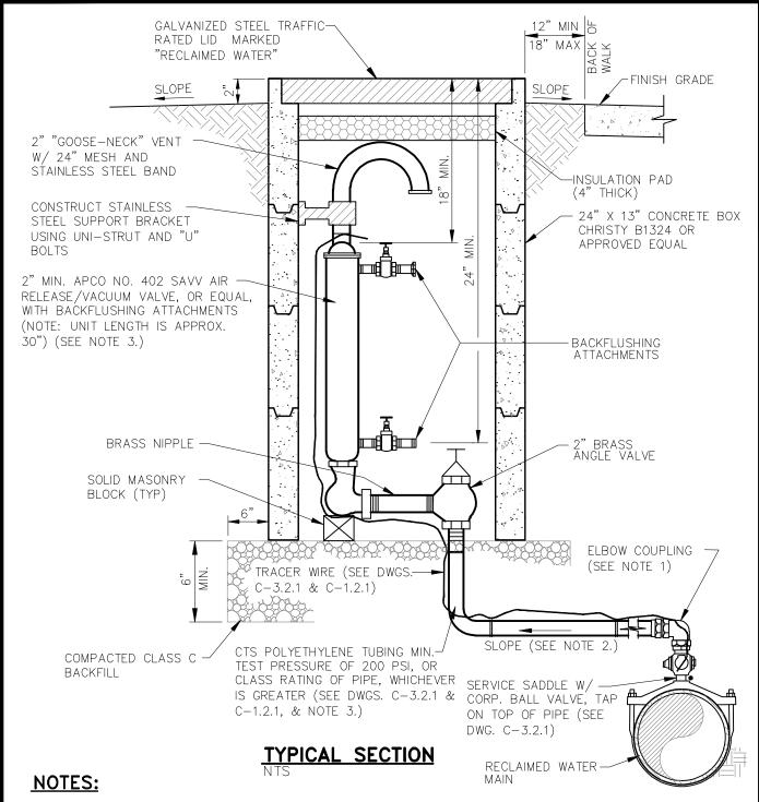
1. AIR RELEASE/VACUUM VALVES SHALL BE INSTALLED OUTSIDE PAVEMENT SECTION. SLOPE GROUND AWAY FROM AIR RELEASE/VACUUM VALVE BOX OR CONSTRUCT MINIMUM HEIGHT CURBING TO PROTECT FROM FLOODING BY SURFACE WATERS.
