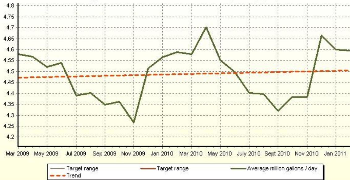
Average Wastewater Reclamation Plant outflow (effluent) (PW)
