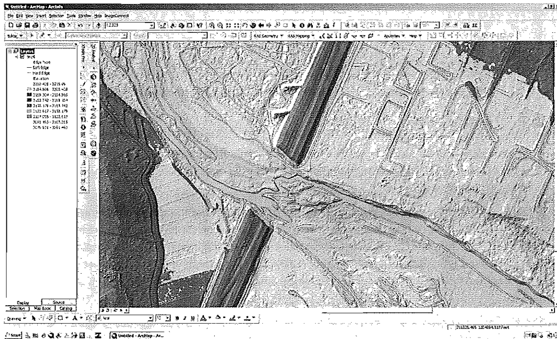
Figure 10: Example bare earth surface terrain missing bridge data
