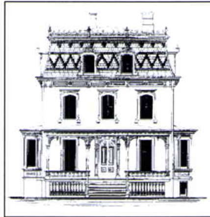
Front elevation of a dwelling published in Supplement to Bicknell's Village Builder . A specification for one of the designs included this direction for the French roof: "Slate the sides of the roof with slate 5 x 12 inches, cornered as shown on elevation, nailed with galvanized nails; all hips and valleys to be flashed with tin in the best manner." (Courtesy of The Athenaeum of Philadelphia)
