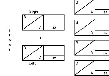
**Replace Tire If The Tread Depth Is Below** 4/32" At Any Point On The Tire
