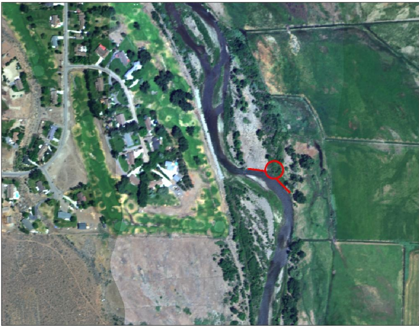
Figure 3.1-3: Example of Channel Migration in Carson Valley (provided by J. Stone, NDEP)
