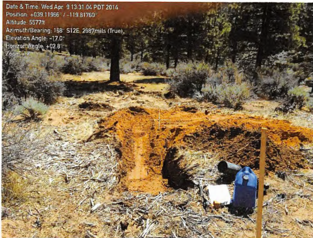
PHOTO 7 – Percolation Test Pit TP – 7.
