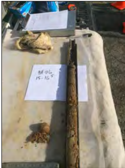
PHOTOGRAPH #5 Typical Mottling Above Saturated Zone at 17 Feet Below Existing Surface.
