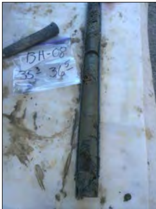
PHOTOGRAPH #5 Typical Mottling Above Saturated Zone at 17 Feet Below Existing Surface.
