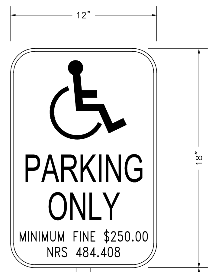
REFER TO CARSON CITY STD. DETAIL C-5.4.2 TRAFFIC SIGN INSTALLATION FOR MOUNTING HEIGHT, POLE, AND ANCHOR ADA SIGN DETAIL NOT TO SCALE
