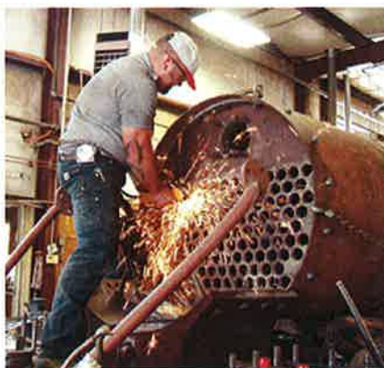
PHOTO BY: WENDELL HUFFMAN; Mort Dolan, restoration specialist at the museum, cuts out the front tube sheet.
