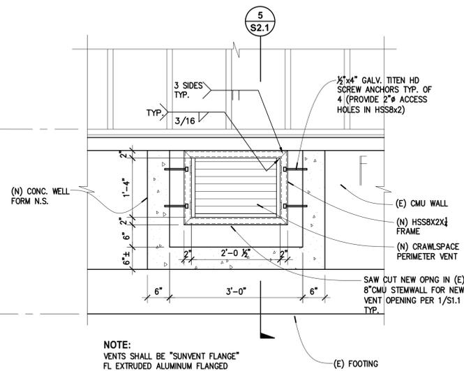
**NEW PERIMETER VENT OPENING- ELEVATION**
