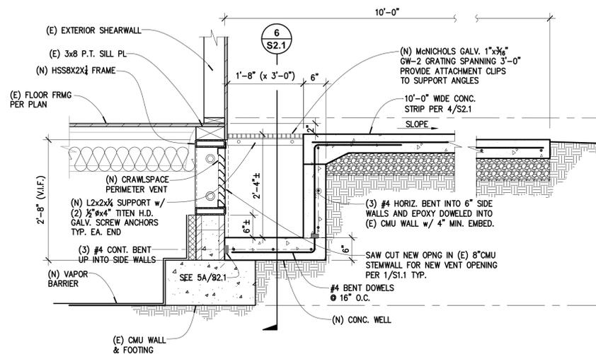
**NEW PERIMETER VENT OPENING- SECTION AT NEW CONC. STRIP**
