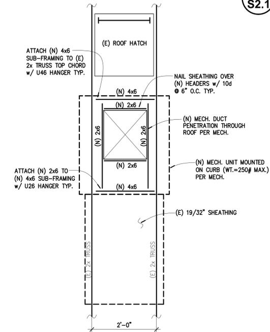
**MECH. SUPPORT FRAMING AT ROOF**
