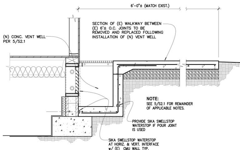
**NEW PERIMETER VENT OPENING- SECTION AT EXIST. WALKWAY**
