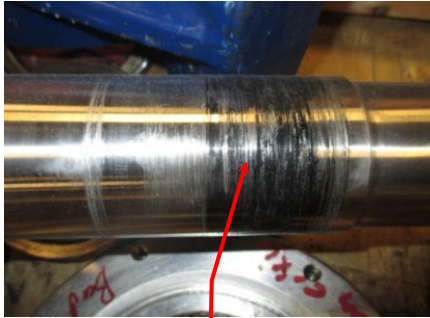
Damaged Feed Pipe
