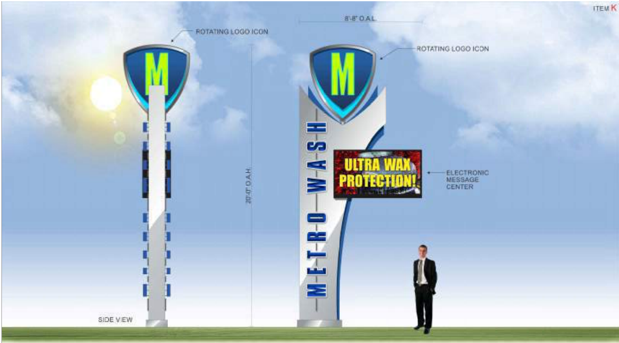
DOUBLE FACE INTERNAL AND HALO-ILLUMINATED PYLON WITH ROTATING ICON AND ELECTRONIC MESSAGE CENTER- SCALE: 3/4" = 1'-0"
