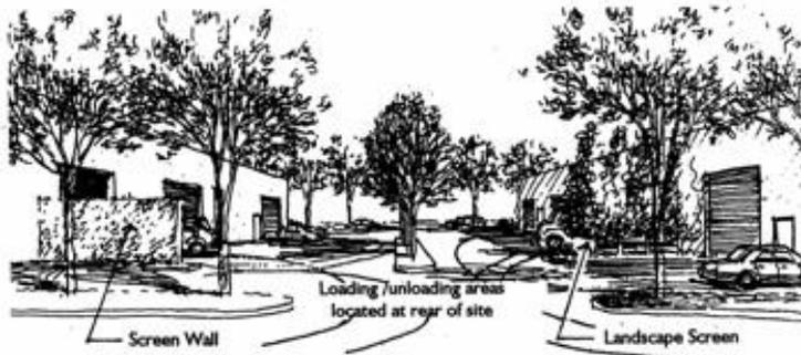
**Typical loading/unloading area screened and oriented away from the street.**
