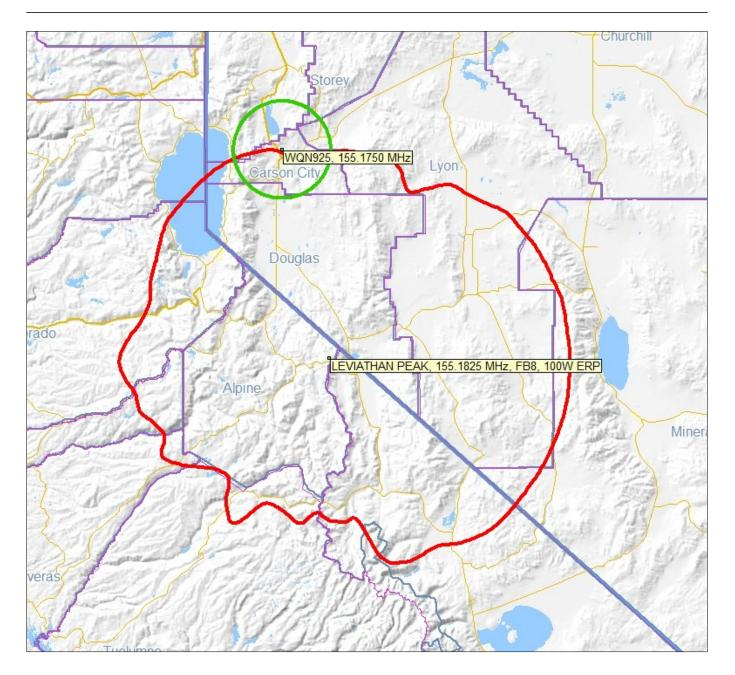
Proposed Frequency: 155.1825 MHz, FB8, Centralized trunked Relay ERP: 100 Watts
