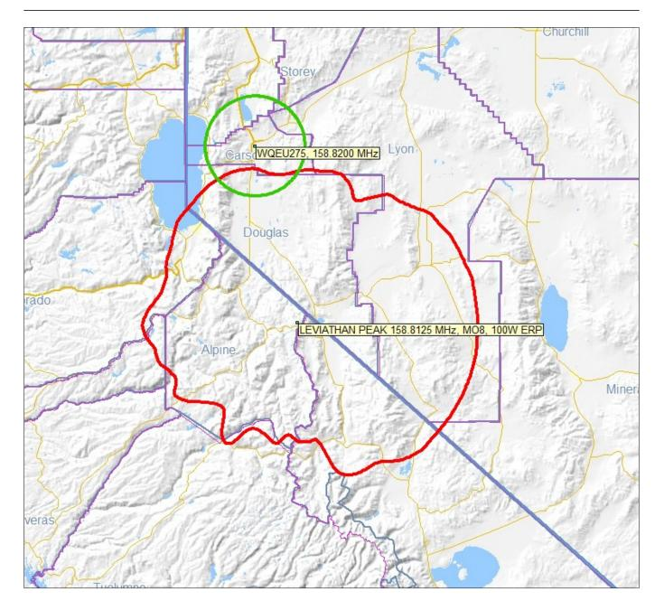
Proposed Frequency: 158.8125 MHz, MO8, Centralized trunked Mobile ERP: 100 Watts
