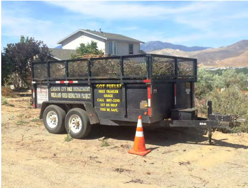
Photo #1 – 7’x12’ Fuels Collection Trailer. Carson City currently has 5 of these trailers which average 1000 lbs. of vegetation per trip.
