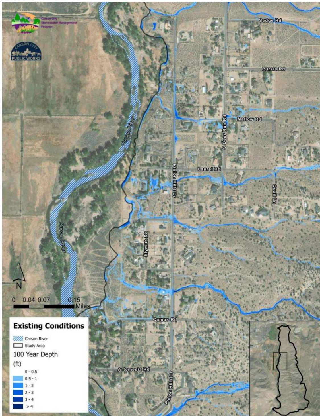
Figure 3-6: Existing Conditions 100-year, 24-hour Flow Depths
