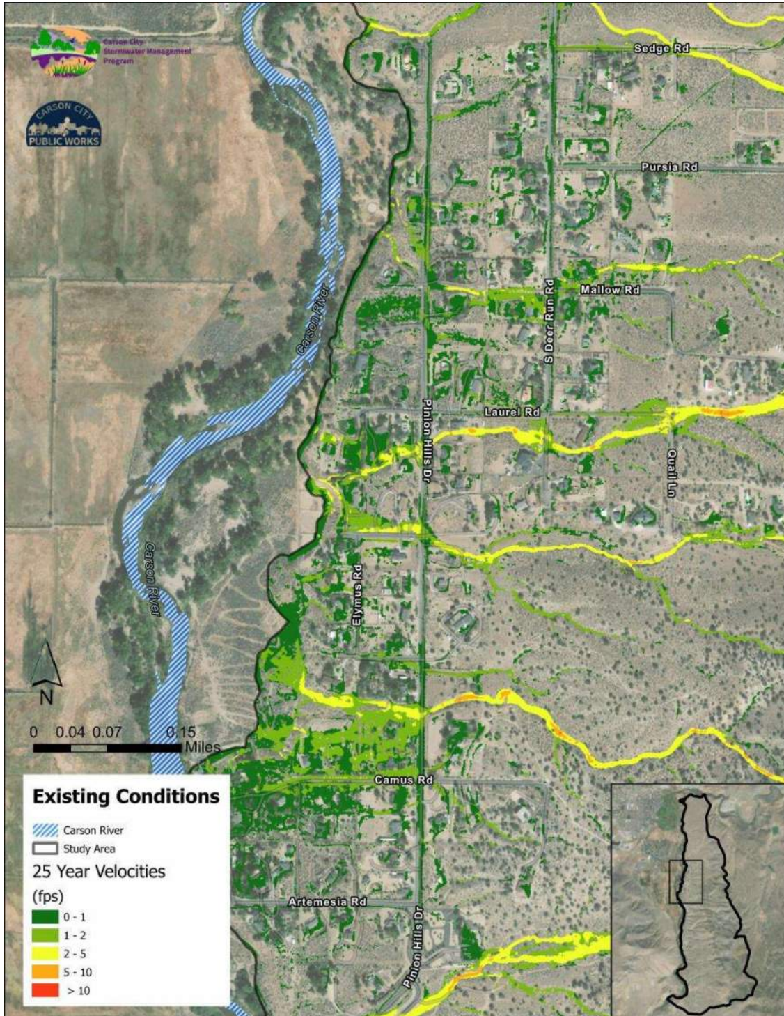
Figure 3-5: Existing Conditions 25-year Velocities
