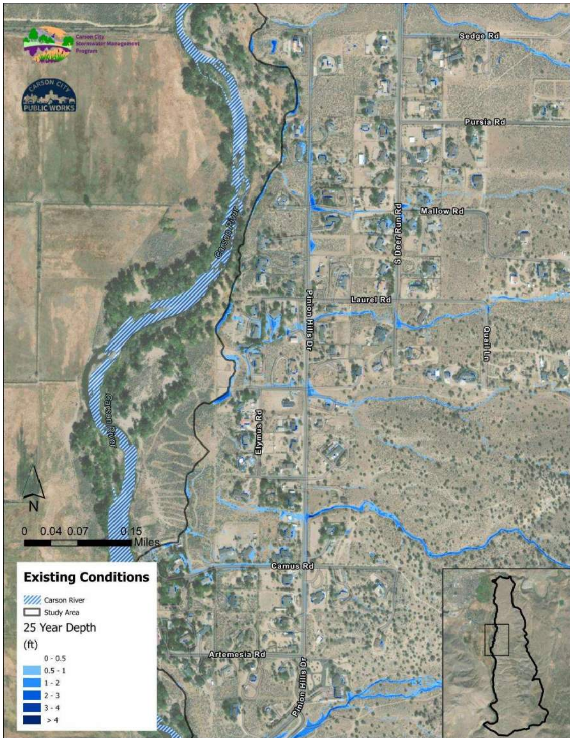
Figure 3-4: Existing Conditions 25-year, 24-hour Flow Depths
