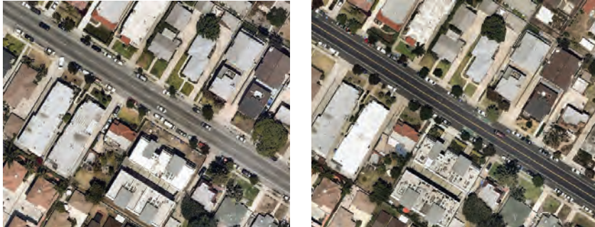
Before-and-after road reconfiguration on Duquesne Avenue in Culver City, CA. General Flow lanes were narrowed to make way for a bike lane while retaining parking.
