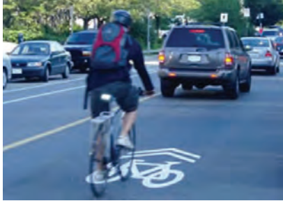
Sharrows also serve as positional guidance and raise bicycle awareness where there is not space to accommodate a full-width bike lane. Center lane markings may or may not be necessary depending on travel lane widths. Narrower two way residential streets (less than 22 ft between parked cars) have a natural traffic calming effect without center turn lanes.
